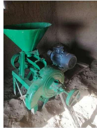
Figure 4: Shea pump kneader with electric motor
